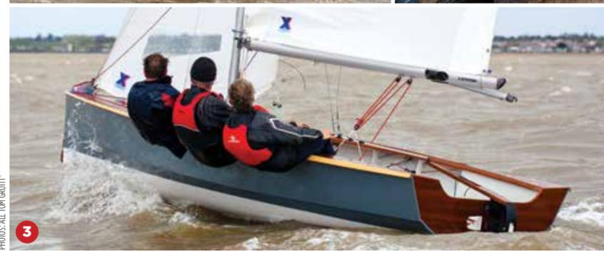
“Marked chines and generous beam contribute to stability, but it's not so wide as to distort the hull shape”
